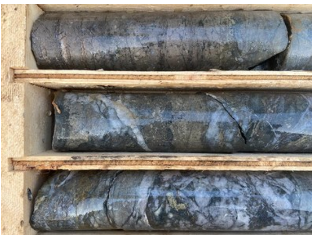
Figure 6: GH-DDH-21-004: 353.9m to 357.4m. (Top row) Massive dark brass coloured pyrrhotite with semi-massive pyrite along margins overprinting an earlier tourmaline-silica breccia. (Middle
