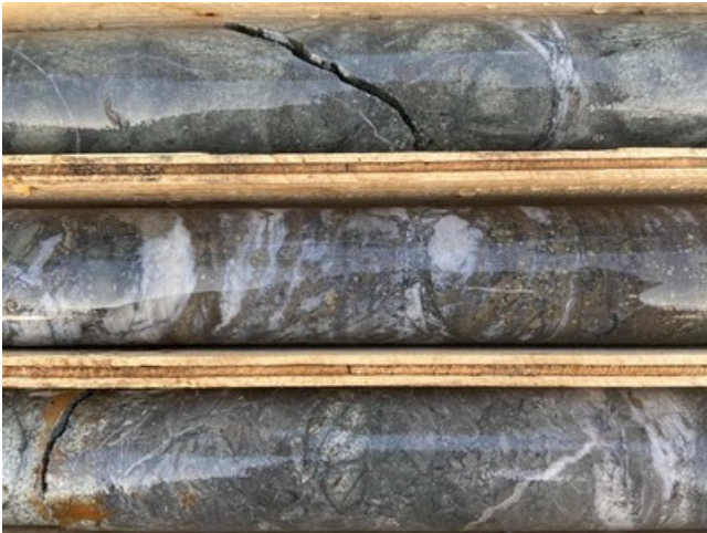
Figure 4: GH-DDH-21-004: 353.9m to 357.4m. Massive pyrite overprinting refractured early quartz veins with a secondary pyrite mineralizing event with brighter coloured blebby pyrite. (CNW Group/Talisker Resources Ltd)
