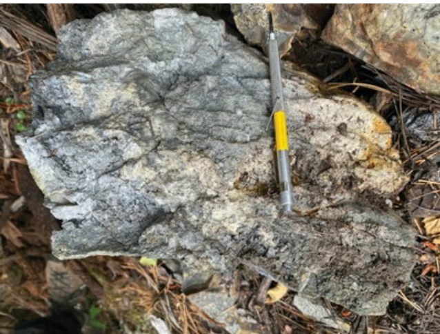
Figure 2C - Photograph of massive sulphide and quartz veining from the Golden Hornet project area (CNW Group/Talisker Resources Ltd)
